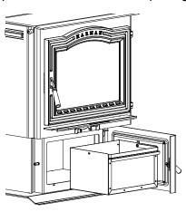
opening the ash door and removing the ash pan, open the bypass damper. Wearing heavy protective gloves, open the ash door and remove the ash pan by pulling it forward by the handle. Close the ash door and damper bypass before taking the ashes outside for safe disposal.
