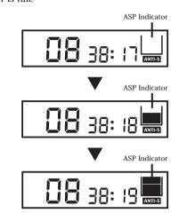
The sound will mute for approximately 1 second while the buffer fills. Once filled the buffer will give approximately 10 seconds of protection against interruption of sound output. If the player is subjected to shocks of over 10 second duration some interruption of sound output will occur. This is normal and to be expected and the sound will resume once the player has stabilized from the shock.
