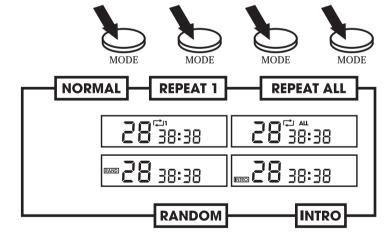
Push MODE button once and is shown in the LCD display, the current track on the disc will be repeated.
