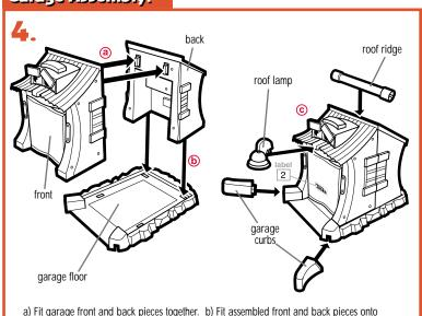
a) Fit garage front and back pieces together. b) Fit assembled front and back pieces onto garage floor. c) Attach roof ridge, roof lamp, garage curbs and label as shown.
