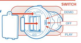
batteries. Replace door and tighten screw.
