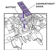
Using a Phillips/cross head screwdriver (not included), loosen screw in battery compartment door. Remove door. Insert 3 x 1.5V "A76" or LR44 size alkaline batteries. Replace door and tighten screw.
