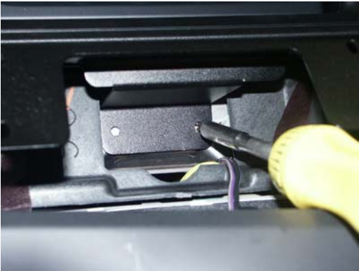
Slide bracket between trim around radio and the trim panel previously removed
