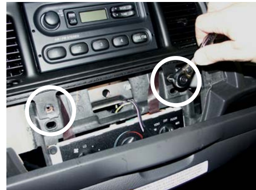
Remove hex head trim screws shown above
