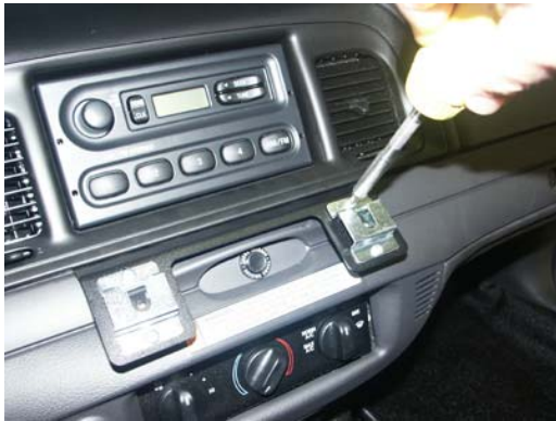
Install microphone clip brackets using #8 x 1/2" machine screws and hex nuts
