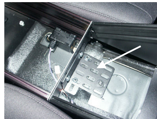
Place console assembly and install extension (#10) for "L" bracket mounting leg on stout console, using OEM hardware.
