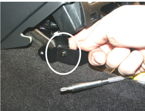
Attach frame support bracket (#4) to vehicle using 10/32 x 1/2" phillips machine screws, washers, and keps nuts
