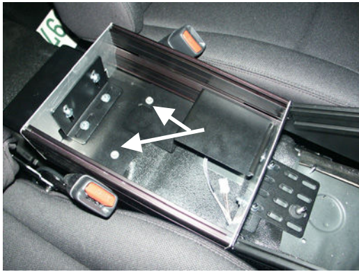
Attach rear floor filler panel (#6) to vehicle using OEM hardware
