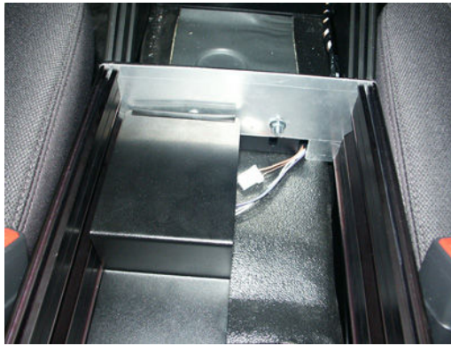
Attach YAW sensor cover panel (#5) to vehicle using front driver side hardware from rear floor filler panel (#6)
