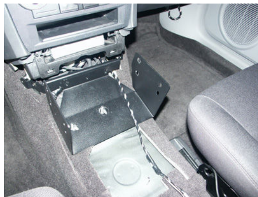
View of installation to this point Note: Be sure OEM wiring is not being crushed by mounting brackets
