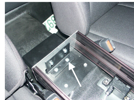
Attach "L" bracket mounting leg (#9) to rear floor filler panel (#6) using 1/4-20 x 3/4" hex bolts and serrated nuts.
