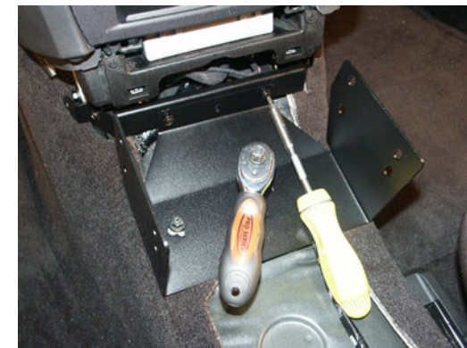
Attach support bracket for stout console (#2) to vehicle and to frame support bracket using OEM hardware and #10 x 1/2" phillips machine screws and washers
