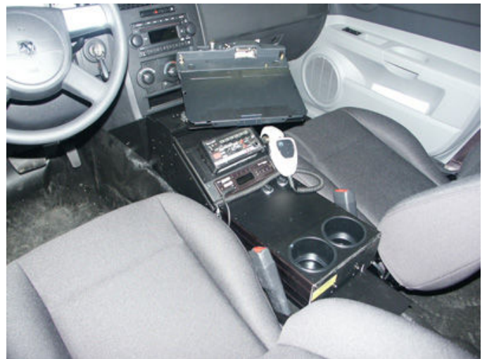
Route wiring and install emergency controls and accessories
