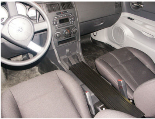
Remove OEM supplied trak. Note: Some hardware is re-used in installation of console
