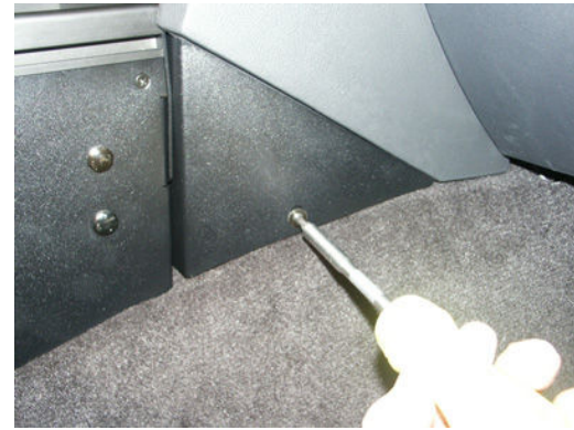
Attach driver and passenger-side wire panels (#7 & 8) to frame support bracket using #10 x 1/2" phillips machine screws and washers.
