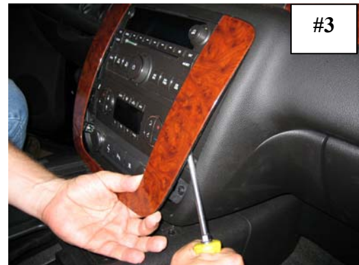
CAREFULLY separate trim bezel from dashboard
