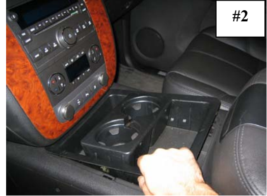
Remove factory cup holder/accessory pocket from console
