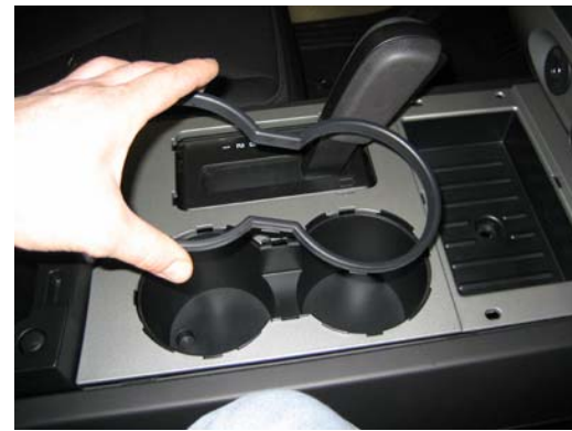
Remove trim from around the cup holders
