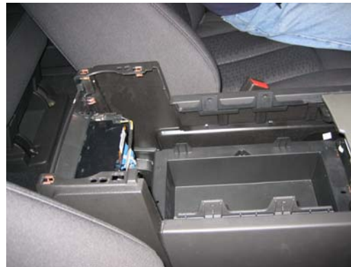
Completely remove the container of the accessory pocket
