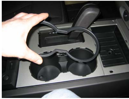
Replace trim panel around factory cup holder
