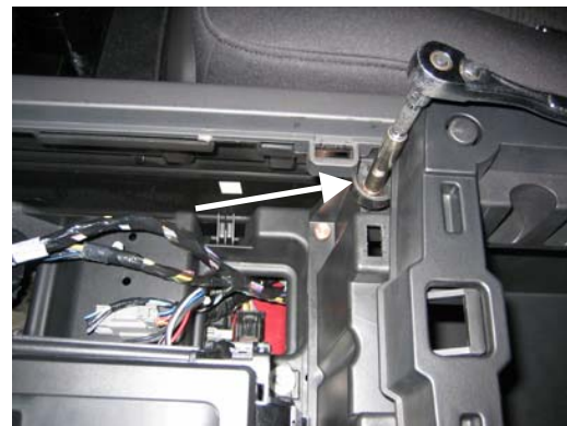
Remove hex head screw from accessory pocket/armrest
