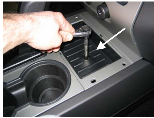
Replace hex head screw on accessory pocket
