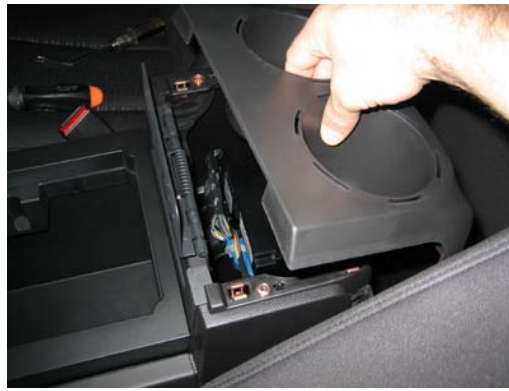
Remove the rear OEM cup holder
