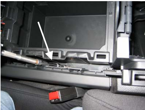
Remove hex head screws holding lower sides accessory pocket
