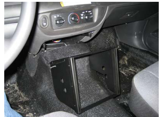
Slide console into ashtray frame slide rails
