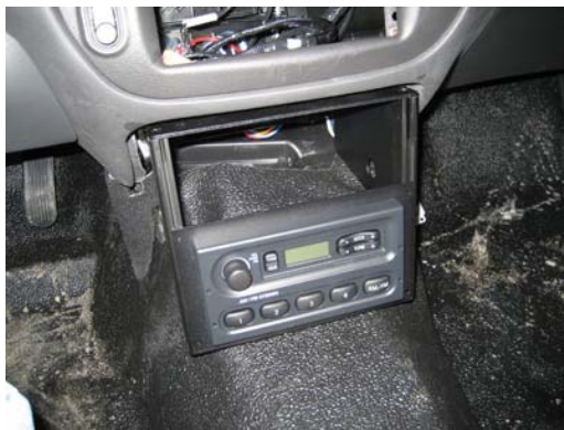
Install AM/FM radio if necessary, as shown above.
