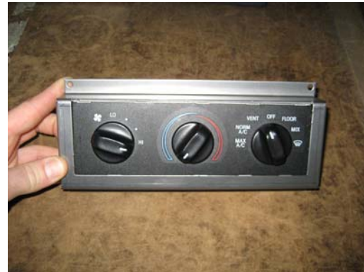
Install HVAC controller into C-EB40-ACV-1P as shown and install into console above AM/FM radio
