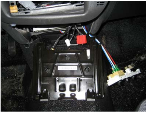
Re-route HVAC controller and the AM/FM radio harness and antenna to the VS console
