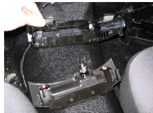
Power point detached from assembly
