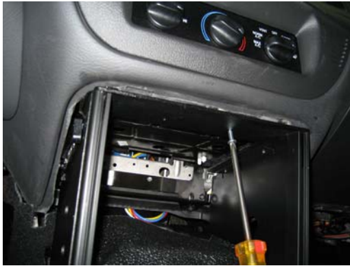
Attach using #10 x 3/4" sheet metal screws.
