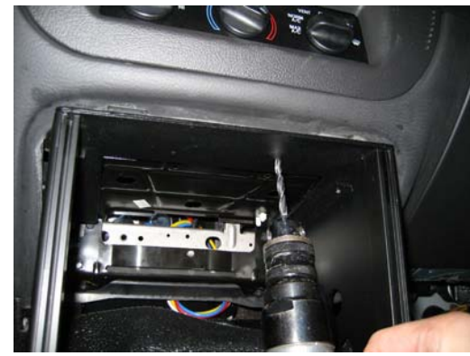
Pre-drill OEM dash using holes in console as a drill template
