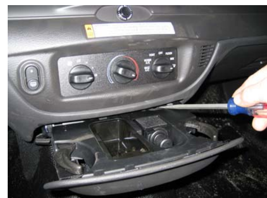
A flat head screwdriver is needed to release the tray from the slide tracks
