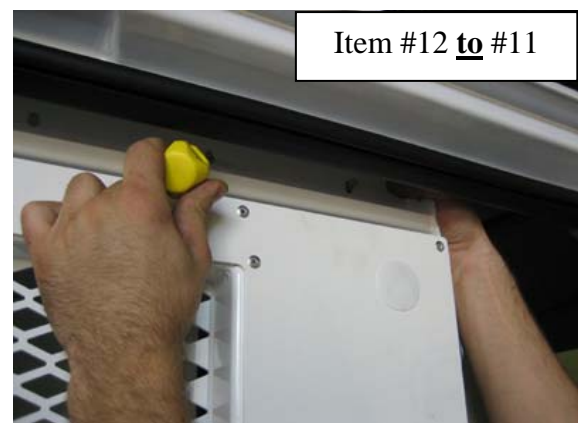
Align 3 rd Compartment Doorframe to 3 rd Compartment Ceiling and loosely attach 1/4" x 3/4" hex head bolts, washers and serrated nuts.
