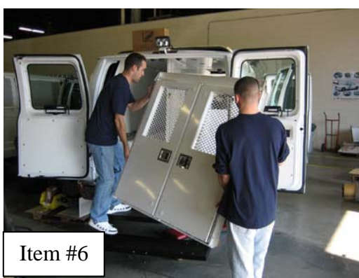
Place Rear Bulkhead Doorframe into vehicle
