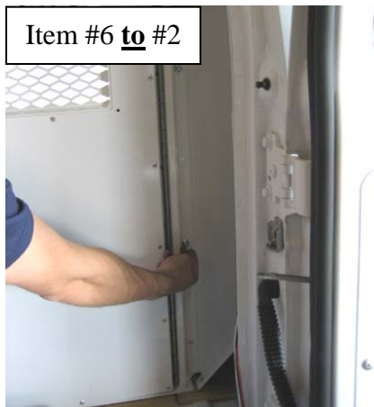
Loosely bolt Rear Bulkhead Doorframe (at the door hinge) to Bench/Wall assemblies using 1/4" x 3/4" carriage bolts, washers and serrated nuts
