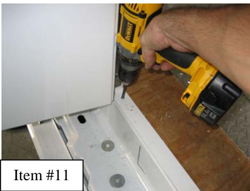
3/8" x 2" hex head bolt, flat washer, fender washer, lock washer, and nut
