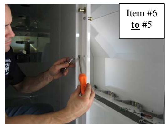
Loosely attach Doorframe to Center divider using #10 x 3/8" flat head machine screws and nylock nuts
