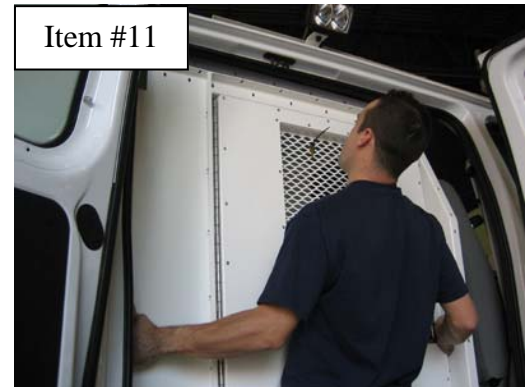
Place the 3 rd Compartment Doorframe assembly.
