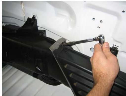
Remove the hex head screws on the intake cover
