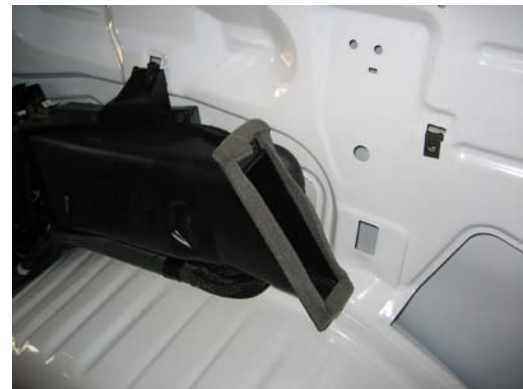
Remove the intake cover. Intake cover will not be re-used.
