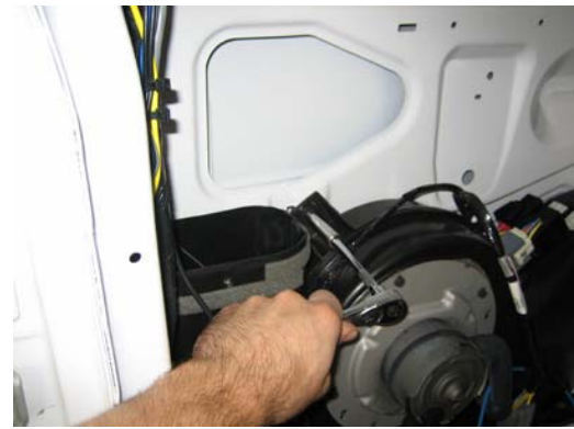
Remove the hex head lag bolt located above the blower motor of the OEM rear HVAC unit
