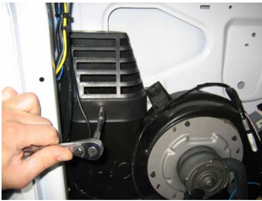
Remove the hex head screw on the vent cover
