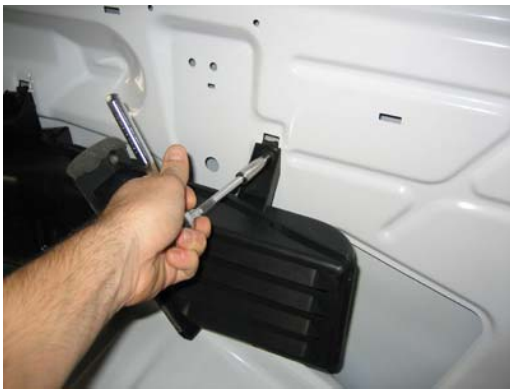
Remove the hex head lag bolt holding the intake cover of the OEM rear HVAC unit
