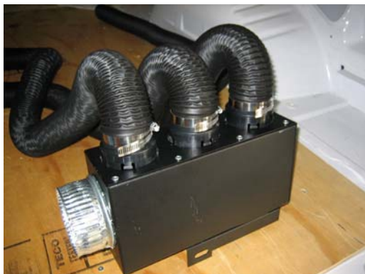
Attach the HVAC hose and clamps to the plenum assembly
