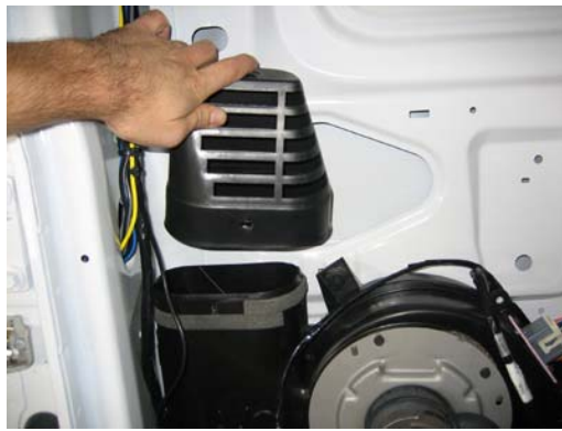
Remove the vent cover completely. It will not be re-used.
