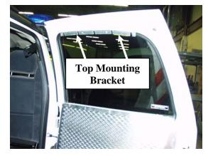
• With top mounting bracket for hinging window guard attached, hinge window up and mark placement for top mounting bracket.
