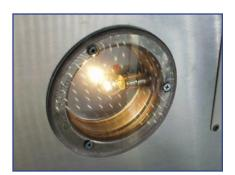
**Dome Lights** Enable officers to see into compartments in preparation for opening doors for loading/unloading.
