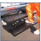
Flip Down Step Optional flip down second step bolts to standard rear step and is designed to help prisoners with leg shackles. Slam latch keeps it in stored position during vehicle operation
