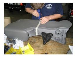
Extend cut line on console sides. Carefully cut off back console section. (Jig saw, Air saw, Dremel or Air drill)
