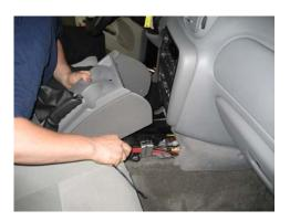
Carefully reinstall front console section. (Reattach Traction Control Plug)
