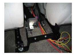
Attach bail bracket onto rear hump brackets with <sup>1</sup>/<sub>4</sub> x <sup>3</sup>/<sub>4</sub> bolts. **Note**: You may need to bend hump brackets slightly forward.
