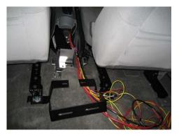
Remove inboard rear seat nuts. (15mm) Place new rear hump brackets on seat studs under seat brackets.
