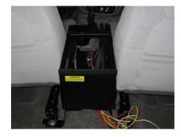
Position console housing as desired and tighten all mount hardware. \*\*Check shift lever in rear position.
