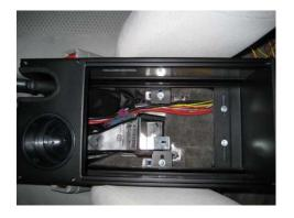
Place new console between seats and position "L" mount brackets onto OEM bracket. Attach with 1/4" x 3/4" bolts.
