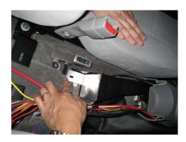
Place duct block off plate in duct opening and screw down with #10 x $\frac{1}{2}$ " sheet metal screw.
