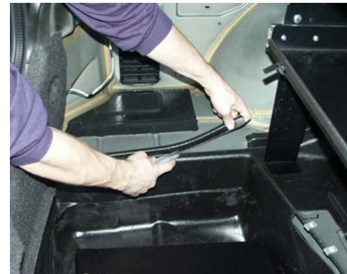
Notch trim as necessary Note: Vehicles w/ carpeted fiberglass trim requires more cutting due to thickness of material, see next page.
