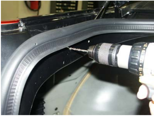
Drill (3) marked holes using 3/16" drill bit
