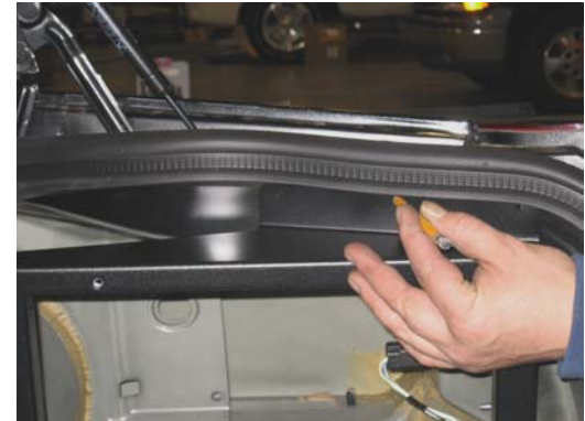
Position Trunk Side Mount and mark (3) holes on top mounting bracket
