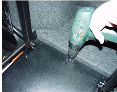
Pre-drill lower mounting holes using 1/8" drill bit and attach with #10 x 3/4" Sheet metal screws
