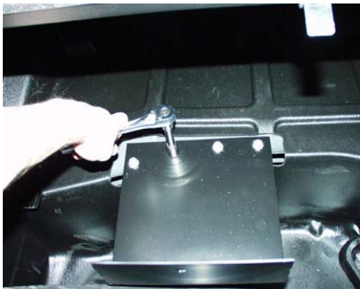
Attach C-STB-CHGR mount, as shown above, using OEM hardware
