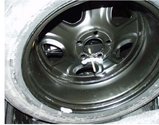
Re-attach "wing" nut onto bolt and tighten.
