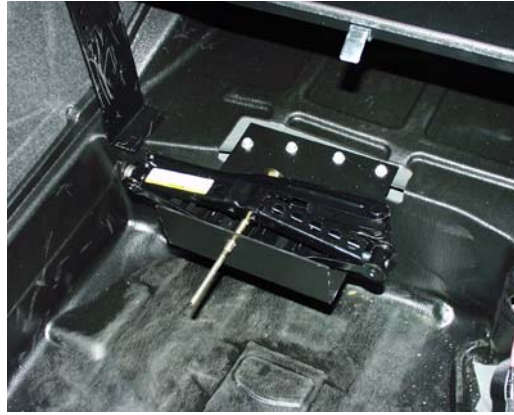
Slide OEM bolt through jack stand, then through C-STB-CHGR.
