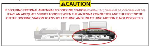
4) Gather all cables to one side and tie off to unused holes on underside of Docking Station.
