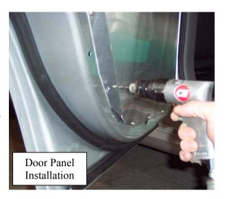
Note: apply wax to screws to avoid screw head from snapping.
