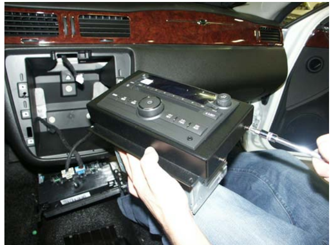
Attach mounting bracket to AM/FM radio and install torx screws to hold radio.
