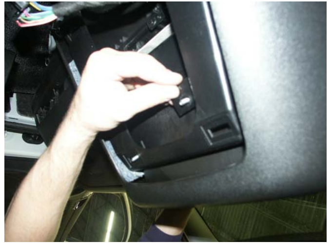
Slide studded mounting plates into the slots used previously to hold the trim panel that contained the lighter plugs.
