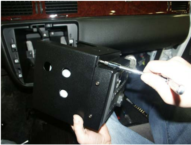
Mount assembled AM/FM radio bracket and radio to main relocation housing.
