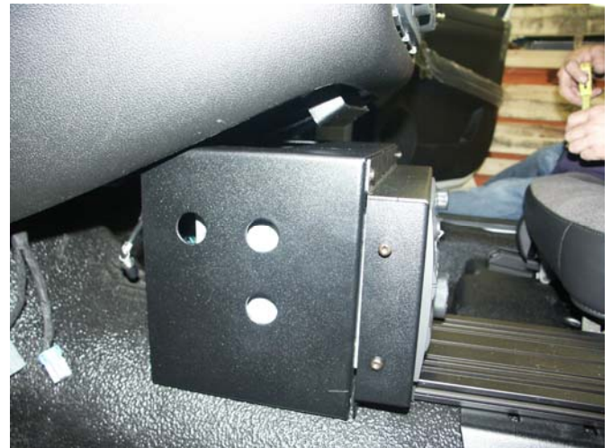
Attach main relocation housing to mounting "hat".
