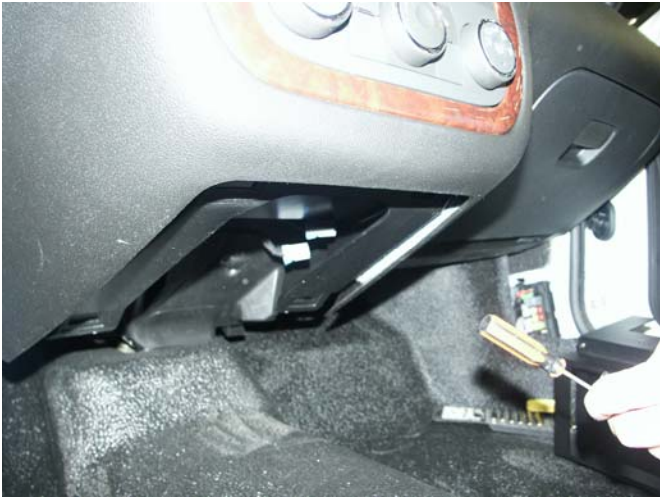
Remove lower plastic trim panel and disconnect cable from lighter plugs.
