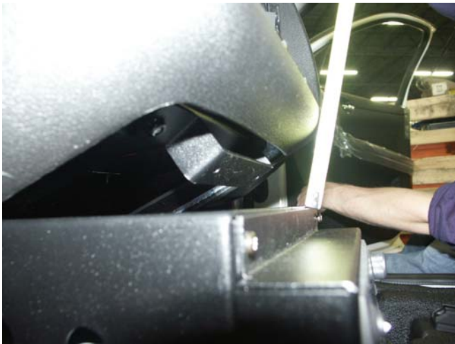
Mount "hat" bracket to studded mounting plates.
