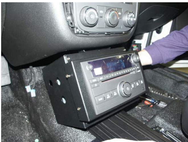
Mount "hat" bracket to studded mounting plates.
