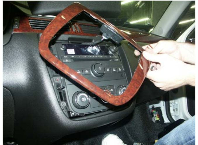
Remove trim around AM/FM radio and thermostat controls.
