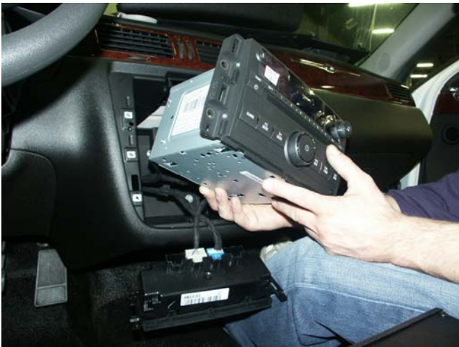
Remove AM/FM radio screws, wire harness and antenna.
