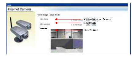
**Camera Name\*** - The camera name will be displayed when the Camera Name field is entered in the Web Configuration setting under **"Configuration"**
