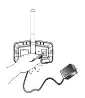
**Note:** Confirm that the device is receiving power by making sure that the "Power" LED is illuminated.
