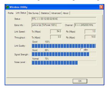
The Link Status page gives you information regarding your current wireless channel, transmit rate (speed) and link/signal quality. You will use this utility to figure out which antenna position results in the best performance and connection.
