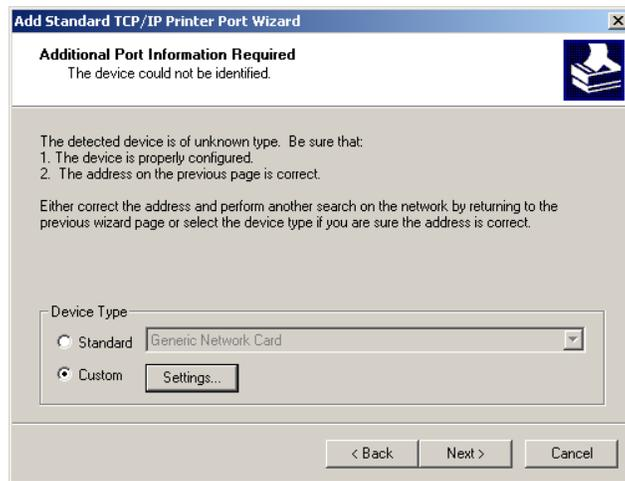
7. In the **Configure Standard TCP/IP Port Monitor** box as shown in the picture above, select “custom device type” and then click **Next**.
