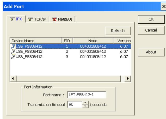
**PID (1): Parallel, PID (2): USB 1, PID (3): USB 2**
