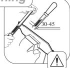
Ensure that the cutterblade is balanced. Use a screw driver with a round shaft to support the cutterblade through its centre hole. Hold the cutterblade horizontal and then release. A balanced cutterblade will remain horizontal.
