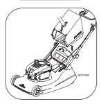
Raise the rear deflector, lower the grassbag between the handlebar and hook in position. Lower the deflector to rest on the grassbag.
