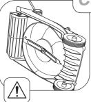
Drain the fuel by running the engine until the fuel tank is empty and the engine stops. **Remove the spark plug lead** and allow the engine to cool. Turn the mower on its left hand side and ensure that the air cleaner side of the engine is uppermost.
