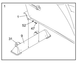
While another person lifts the Rear Frame (3), attach the Rear Stabilizer (10) to the Rear Frame with two M8 x 25mm Button Screws (47) and two M8 Split Washers (52).
