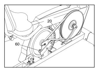
Next, turn the indicated M8 Nylon Locknut (60) until the Drive Belt (20) is properly tightened. Then, reattach the right side shield.
