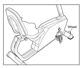
If the exercise cycle rocks slightly during use, turn the leveling feet under the rear stabilizer to eliminate the rocking motion.
