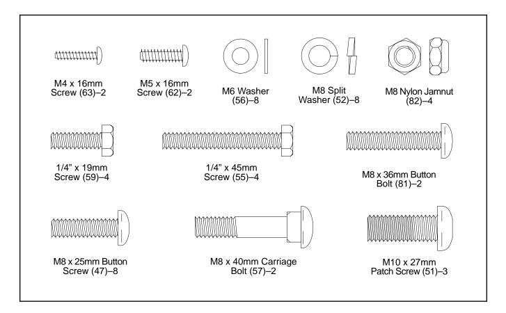
Identify the Front Stabilizer (9), which has Wheels (31) attached to it. While another person lifts the front of the Frame (1), attach the Front Stabilizer to the Frame with two M8 x 25mm Button Screws (47) and two M8 Split Washers (52).
