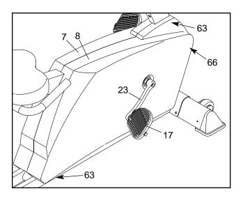
Next, locate the Reed Switch (64). Turn the Right Crank Arm (23) until the Magnet (46) is aligned with the Reed Switch. Loosen, but do not remove, the indi-
