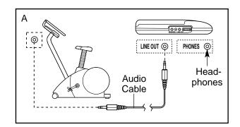
B. Plug one end of a 1/8" to 1/8" stereo audio cable (available at electronics stores) into the jack beneath the console. Plug the other end of the cable into a 1/8" Y-adapter (available at electronics stores). Plug the Y-adapter into the PHONES jack on your CD player. Plug your headphones into the other side of the Y-adapter.
