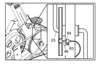
cated M4 x 16mm Screw (63). Slide the Reed Switch slightly closer to or away from the Magnet. Then, retighten the Screw. Turn the Right Crank Arm for a moment. Repeat until the console displays correct feedback. When the Reed Switch is correctly adjusted, reattach the right side shield and the right pedal.
