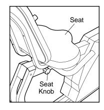
the seat knob is not loosened enough, it may scratch the frame). Next, pull the seat knob, slide the seat to the desired position, and then release the seat knob. **Move the seat back and forth slightly until it locks into place.** Then, turn the seat knob clockwise to tighten it.
