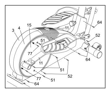
Next, remove the four Screws (51) from the right Pedal Disc (15), and slide the Pedal Disc off. Remove all Screws (52, 64) from the Right Side Shield (4) and the two Screws (77) from beneath the Pedal Disc, and remove the Right Side Shield. Remove all Screws (52) from the Left Side Shield (3) and remove the Left Side Shield.
