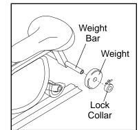
amount of weight on each side of the weight bar. The total combined weight of the user and added weights should not exceed 300 pounds.
