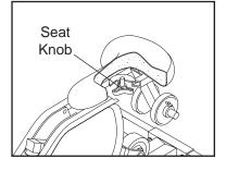
the knob. To determine if the seat is properly adjusted, sit on the seat and pull the handlebar as close as possible to your stomach. Your legs should be almost straight, but your knees should not be locked.
