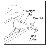
on each side of the weight bar. The total combined weight of the user and added weights should not exceed 300 pounds.
