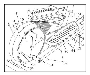
Next, remove the four Screws (51) from the right Pedal Disc (15), and slide the Pedal Disc off. Remove all Screws (52, 64) from the Right Side Shield (4) and the two Bolts (75) from beneath the Pedal Disc, and remove the Right Side Shield (4). Remove all Screws (52) from the Left Side Shield (3) and remove the Left Side Shield.
