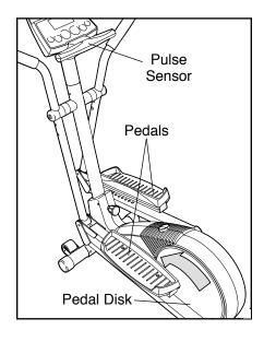
tion. It is recommended that you move the pedal disks in the direction shown by the arrow; however, for variety, you may turn the pedal disks in the opposite direction.
