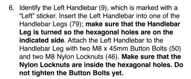
Repeat this step for the Right Handlebar (not shown) and the other Handlebar Leg.
