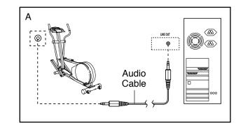
B. Plug one end of a 1/8" to 1/8" stereo audio cable (available at electronics stores) into the jack beneath the console. Plug the other end of the cable into a 1/8" Y-adapter (available at electronics stores). Plug the Y-adapter into the PHONES jack on your computer. Plug your headphones or speakers into the other side of the Y-adapter.
