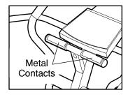
pulse sensor, place your hands on the metal contacts. Your palms must be resting on the upper contacts and your fingers must be touching the lower contacts. Avoid moving your hands. When your pulse is detected, the heart-shaped indicator below the right display will light, one or two dashes (--) will appear, and then your heart rate will be shown.
