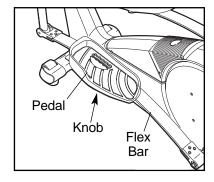
pedals forward or backward to the desired position, and then retighten the knobs. Make sure that both pedals are in the same position.
