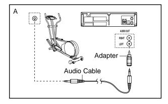
B. Plug one end of the audio cable into the jack beneath the console. Plug the other end of the cable into the adapter. Plug the adapter into an RCA Y-adapter (available at electronics stores). Next, remove the wire that is currently plugged into the AUDIO OUT jack on your VCR and plug the wire into the unused side of the Y-adapter. Plug the Y-adapter into the AUDIO OUT jack on your VCR.
