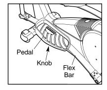
pedals forward or backward to the desired position, and then retighten the knobs. Make sure that both pedals are in the same position.
