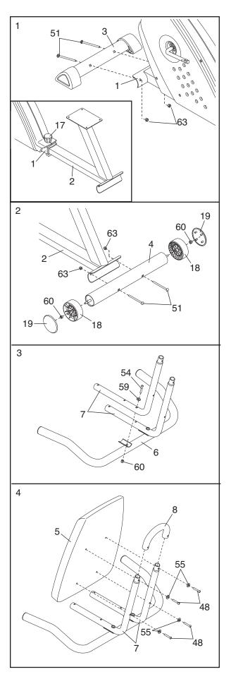
5. Have another person hold the Seat Frames (7) under the Rear Frame (2) as shown. Attach the Seat Frames and the Seat (12) to the Rear Frame with four M6 x 42mm Button Screws (49) and four M6 Washers (55).
