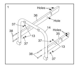
2. Raise the Left Upright (35) and the Right Upright (36) to the position shown. Insert the Reed Switch Wire (6) into the top of the Left Upright and pull it out of the indicated hole.
