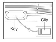
In an emergency, the key can be pulled from the console, causing the walking belt to slow to a stop. Test the clip by carefully taking a few steps backward; if the key is not pulled from the console, adjust the position of the clip.
