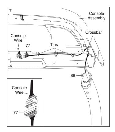
Set the console assembly on the brackets on the Left and Right Uprights (88, not shown). Be careful not to pinch any wires.
