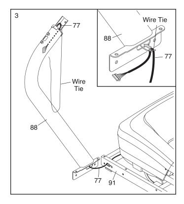
Hold the Left Upright (88) against the Base (91). Be careful not to pinch the Upright Wire (77) or the Ground Wire (90). Insert two 3/8" x 2 3/4" Patch Screws (7) and two 3/8" x 1 1/4" Patch Screws (8) with two 3/8" Star Washers (13) into the Left Upright.
