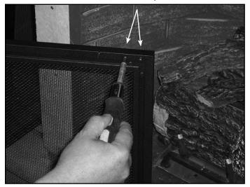
5. Place the hinge on the bottom of left door over the pin and align hole in hinge to top of pin.
