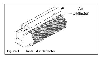
**Note:** Novus appliances do not require the use of the air deflector. Attach the green ground wire with the screw in the existing hole.
