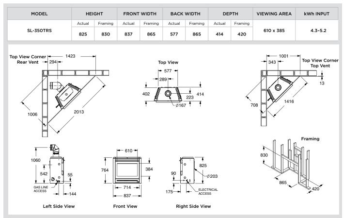
Dimensions above are in millimeters and for reference only. We recommend measuring individual units at installation. Assumes the use of 13mm gyprock.
