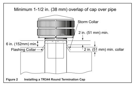
Position the round termination cap over the uppermost chimney section and snap-lock it into position.
