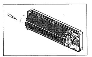
Push right carefully in order to unhook the tabs on the right side of the chassis and pull the evaporator toward you.
