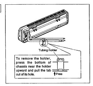
4. Insert the pipings, power supply cord and connecting cable into the piping hole.
