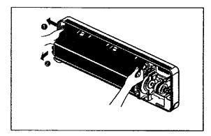
Push right carefully in order to unhook the tabs on the right inside of the chassis and pull the evaporator toward you.
