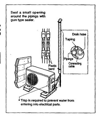
In case of the Outdoor unit being installed above position of the Indoor unit.
