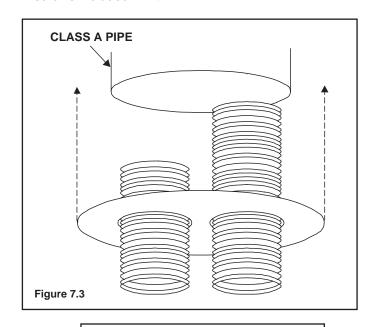
To help eliminate cold air drafts, it may be necessary to place noncombustible insulation around the flues as they go though the damper. **Note**: The LINK-DV4-30B system REQUIRES this insulation.
