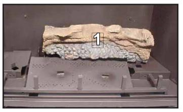
**LOG #1 (SRV339-701):** Place log #1 in the back on the insert. Locate the left end of the log over the center of the pilot and the back side of the left end flush with the back of the pilot bracket. Pull the right end of the log forward until it touches the tab in the base pan.
