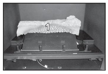
**LOG #1 (SRV349-701):** Place log #1 in the back of the insert. Locate the legs of the log outside the 3/8" tabs to either side of the burner. Pull the log forward until the log is stopped by the back edge of the burner.
