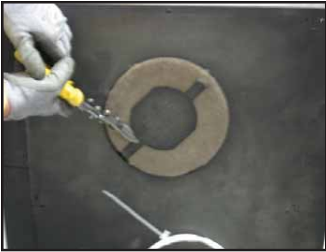
Figure 9.5 Cut the metal retaining band.
