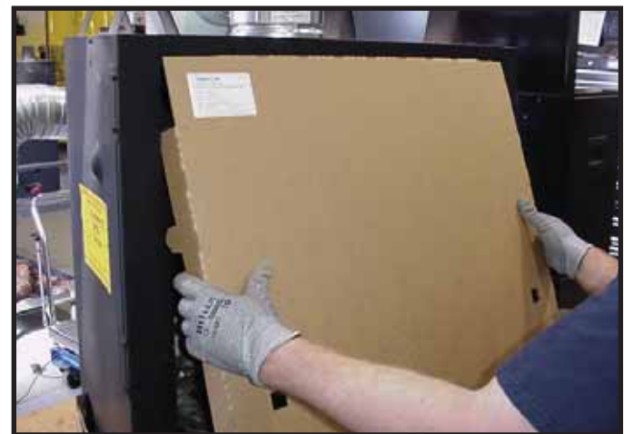
Figure 13.4 Installation of Splatter Guard
