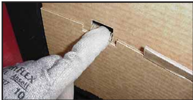
Figure 13.9 Securing Tabs Inside Front of Splatter Guard
