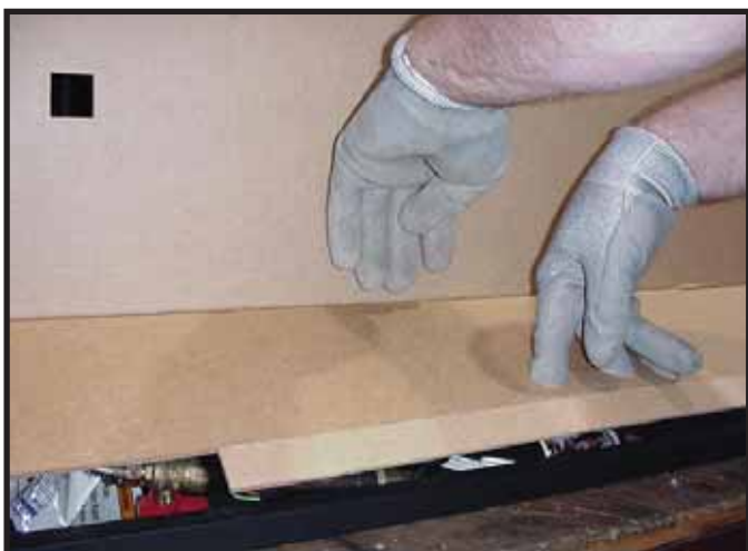
Figure 13.8 Opening Lower Access Panel
