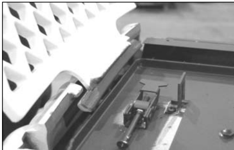
Figure 8.22 Gently lift cast top off of unit and set aside.
