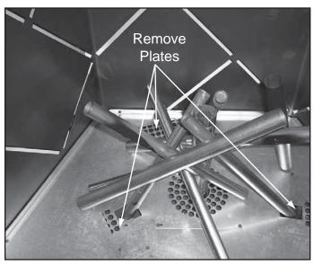
Figure 15.3 Remove Three Plates
