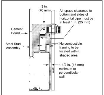
Figure 8.1 Horizontal Venting Clearances To Combustible Materials
