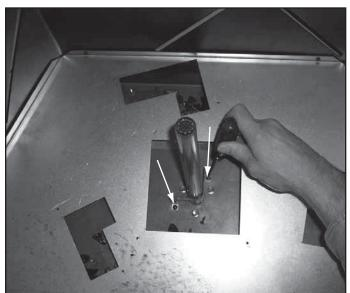
Figure 3.11 Remove Center Burner Tube
