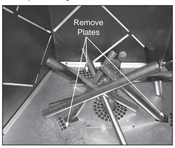
Figure 3.8 Remove Three Plates
