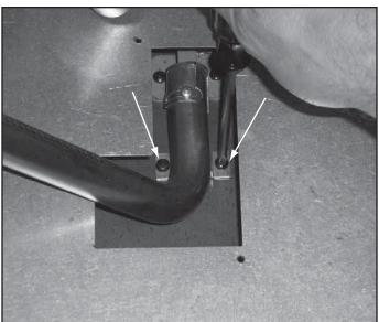
Figure 3.9 Remove Outside Burner Tubes
