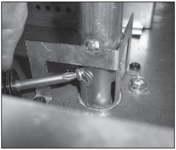
Figure 15.7 Adjust Center Burner Tube Air Shutter
