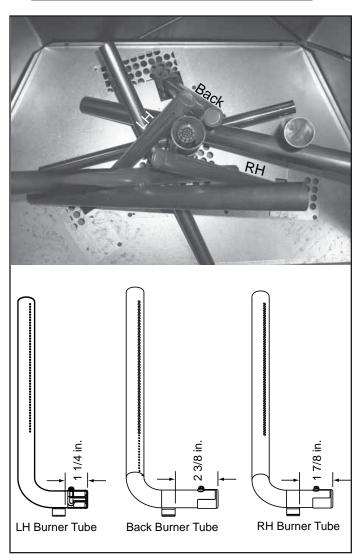
Figure 3.7 Burner Tube ID
