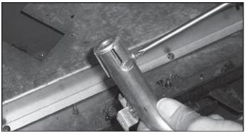
Figure 15.5 Outside Burner Tube Air Shutter Adjustment
