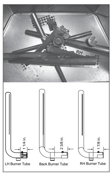
Figure 15.2 Burner Tube ID
