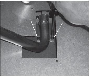
Figure 15.4 Remove Outside Burner Tubes
