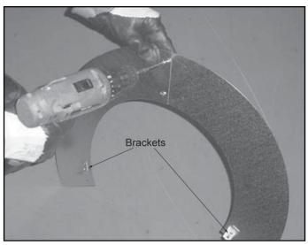
Figure 10.13 Assembling the Storm Collar
