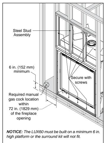
Figure 9.1 Proper Positioning and Securing of an Appliance
