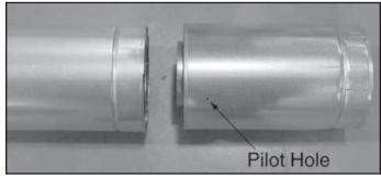
Figure 10.5 Slip Section Pilot Holes
