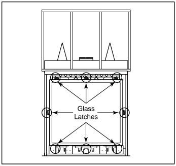
Figure 15.1 Glass Assembly Removal
