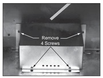
Figure 3.12 Remove Pilot Shield
