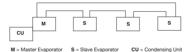
Each Beacon II board power is supplied by a transformer in the evaporator on which it is mounted. Do not run any 24 VAC wires between Beacon II boards on the evaporators.
