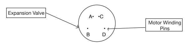
For valve size 29320003 and 2930004, the resistance measured between pin locations A and B or C and D should be approximately 336 Ohms when valve is at 75°F.
