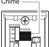
Figure 5 - Determining Correct Jumper Position (Back of Push Button)
