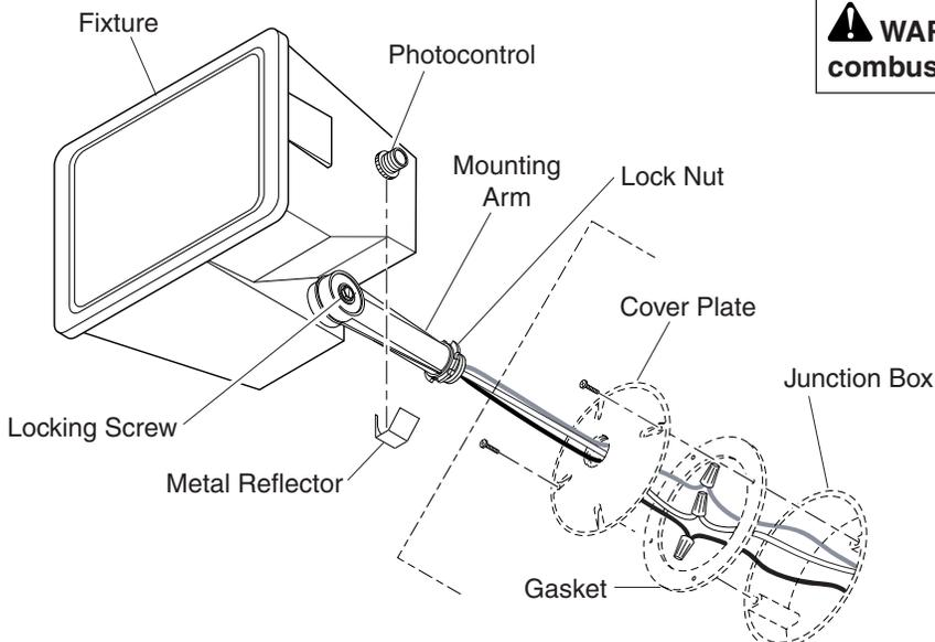
2. Connect the fixture wires to the junction box wires (**black to black, white to white, and the fixture ground wire to the junction box ground wire**). Secure with the wire connectors provided.
