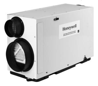
Duct Sizing: Use minimum 10-in. diameter round for duct lengths up to 25 ft. Minimum 12-in. required for lengths longer than 25 ft. Duct branches from the main inlet/exhaust should be minimum 10-in. round for 2-3 branches, and 12-in. round or larger for 4 branches or more.
