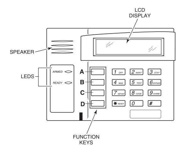
**IMPORTANT!:** When using the keypad to enter codes and commands, sequential key depressions must be made within 3 seconds of one another. If 3 seconds elapses without a key depression, the entry is aborted and must be repeated from its beginning.
